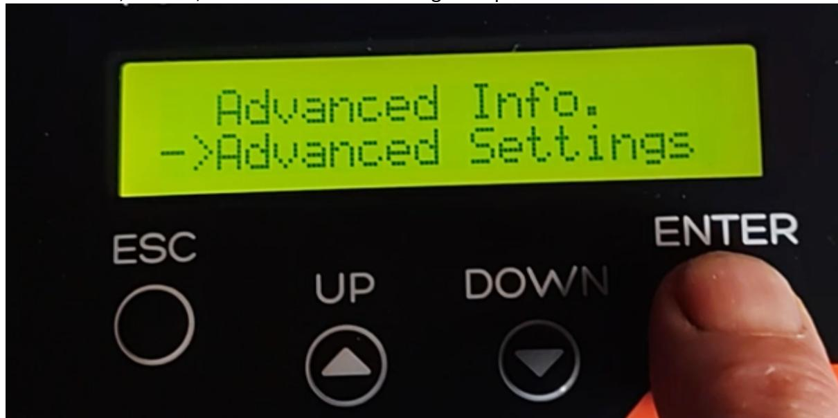
The “password” is 0010 and so you press down 3 times to reach the third digit and press up to set this digit to 1
