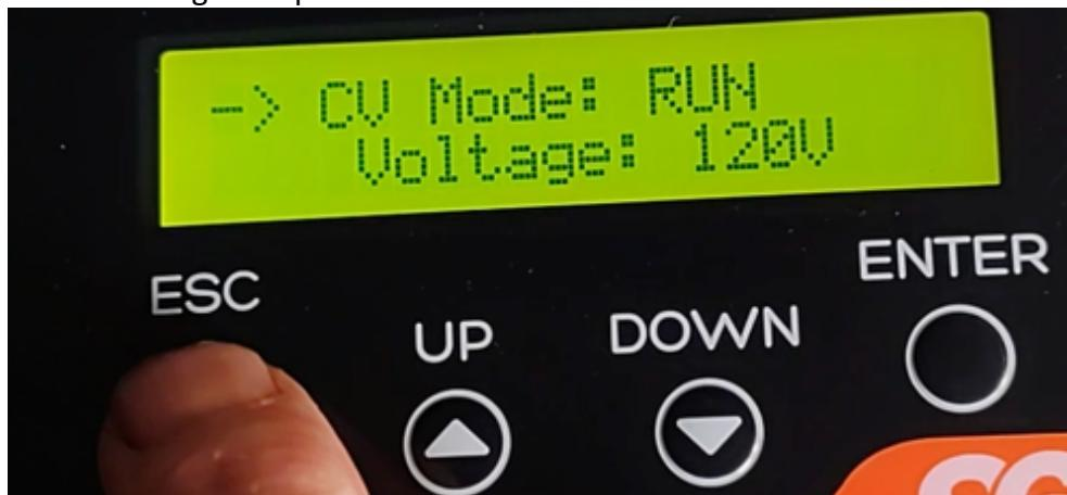
Press UP to return to the top line, set this to “RUN” and press ESC again to confirm the settings.
