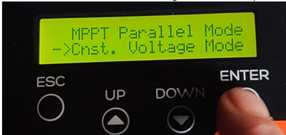
Press DOWN once to reach the line Set Voltage and then use the UP and DOWN keys to select a voltage and press ESC to set that choice.
