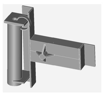
6. When it is well positioned, <u>weld the top (6) and</u> <u>bottom (7) brackets of the yaw pipe to the alternator</u> <u>frame (piece 1).</u>
