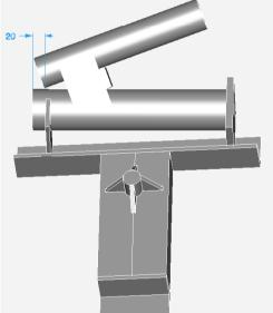
Finally add the two side pieces to strengthen the hinge pipe. These are pieces 10 and 11, made from flat-bar. The neatest way to cut them is square at one end and angled at the other with sides 85 and 60 mm long. One piece  $50 \times 6 \times 145$  mm long could be angle cut at the centre to produce the two pieces you need.
