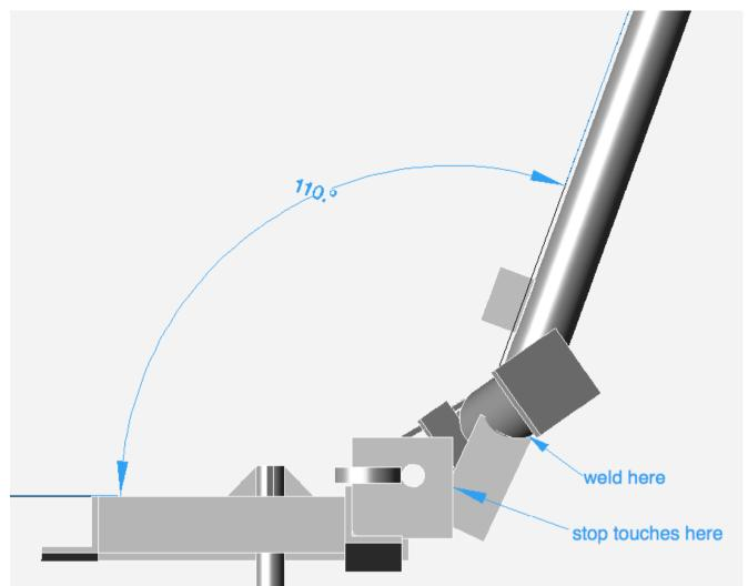
Hold the tail at a 110 degree angle to the back of the alternator frame. A cardboard template with the required angle can be a useful tool to help find the correct position. Plus or minus 3 degrees is fine. Then hold the low end stop (piece 16) against the tail hinge pipe (piece 13) and swing it into contact with the yaw pipe (piece 5).
