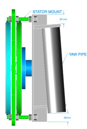
Next is to weld the brackets to the inside of the angle (piece 1) of the alternator frame. Position the yaw pipe centrally so that there is about 30 mm of angle projecting top and bottom.
