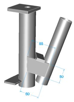
2. Once you are satisfied that the pipes are correctly aligned to each other, weld the 30 mm cross-piece to the yaw pipe, remove the vice grips and weld the bottom of the hinge pipe to the yaw pipe.
