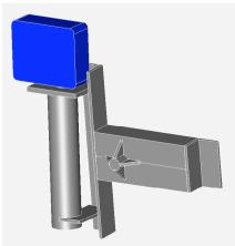
Do not mount this in direct contact with the steel. Fit plastic packing between the box and the yaw cap plate. Bolt together with stainless steel fixings. Position the box directly above the hole in the yaw cap so that the tower wiring enters the box directly and is suitable anchored within the box to support its weight.
