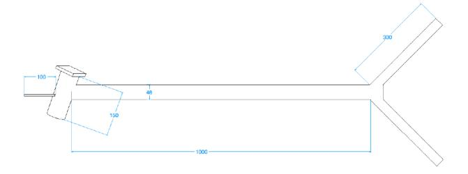
Cut the tail boom out of 1  $\frac{1}{2}$ " pipe 1000 mm long. Measure a point 15 mm from the end of the boom and cut at 45 degrees as shown on the right.
