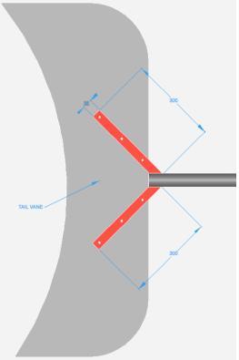
These brackets will be welded on the top and bottom of the tail boom (piece 12) to support the tail vane.
