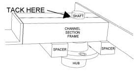
5. <u>Weld the shaft</u> as strongly as possible on both sides, whilst protecting the machined surfaces of the shaft from weld spatter. You can protect it by slipping a metal sleeve over it, or wrapping with a wet rag or covering with copper grease.
