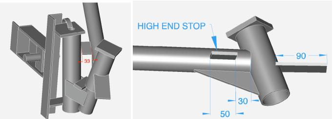
Cut out the high end stop (piece 17) 33 mm long. This is to be welded to the side of the tail boom such that it will contact the yaw pipe (piece 5) when the tail is lifted to its fullest extent.
