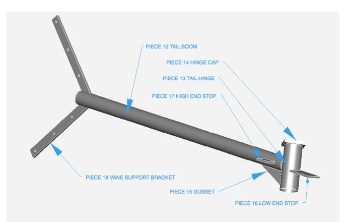
Start off by welding the cap onto the tail hinge pipe (pieces 13 and 14). The hinge pipe (piece 13) is 150 mm length of  $1 \frac{1}{2}$  pipe.
