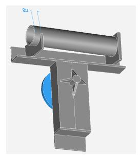
When preparing the stator to mount on the frame it will be useful to be able to drill the stator using the frame itself as a template. So allow enough clearance for a drill to pass through the frame from behind.
