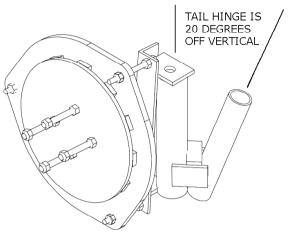
Piece 8 is the inner pipe of the hinge, 250 mm long.
