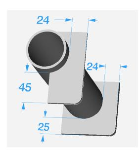
The view above shows the underside of the cap. The pipe is welded on top of it. Note that the pipe must be 24 and 25 mm away from the two edges that will be welded to the alternator frame.
