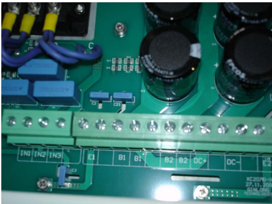
**Figure 5: Connections Terminals of Controller**
