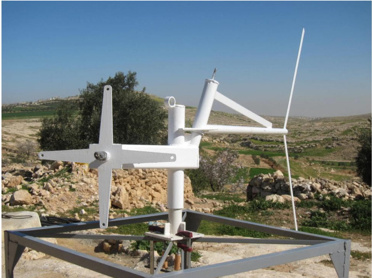
Turbine frame painted and tail with stops assembled at normal tail angle
