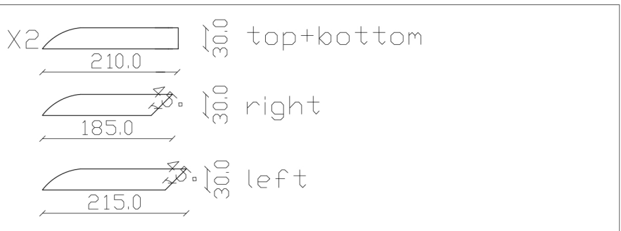
stator ribs 6mm thick
