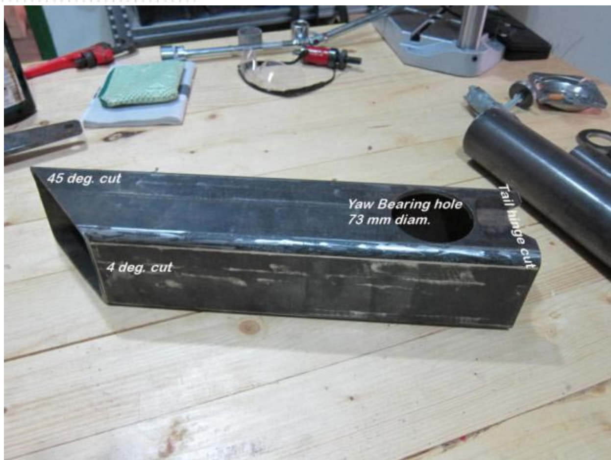
Image of the main frame ready for welding: 45 dg is cut, 4 deg is cut, yaw bearing hole is drilled and the circular notch for the tail hinge axis is cut.
