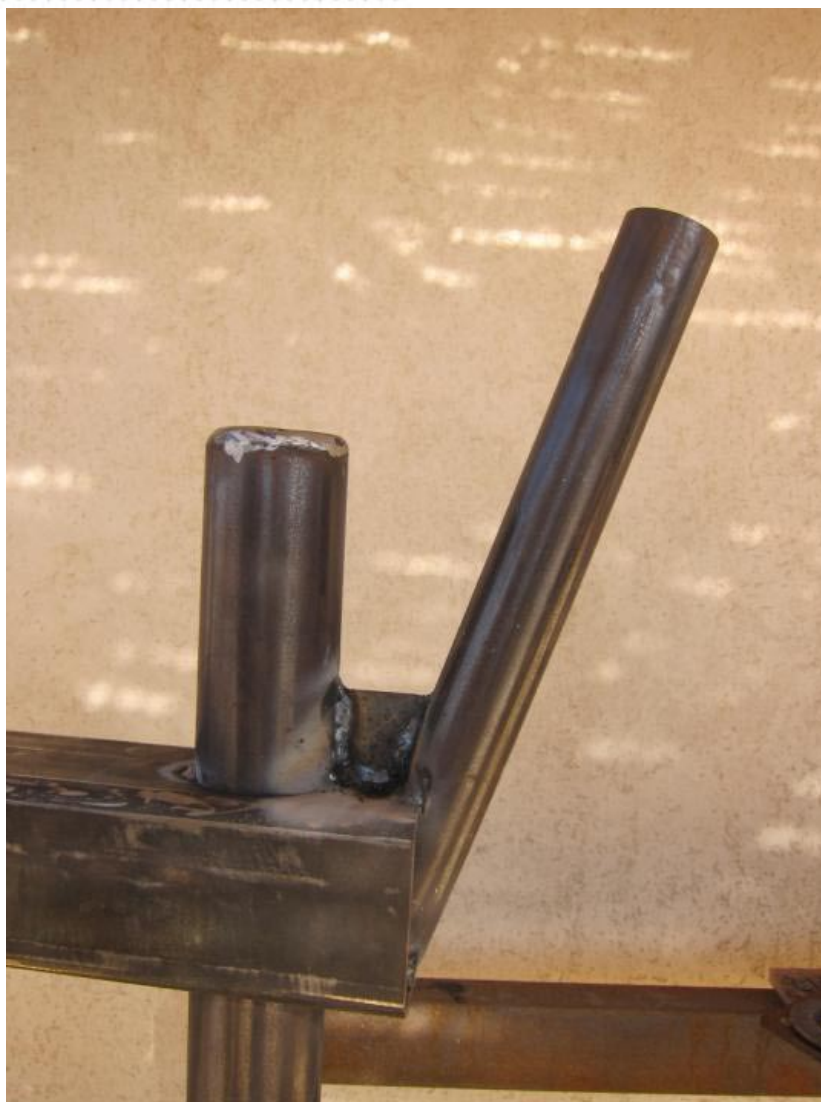
Fourth step: Weld the tail hinge axis bracket
