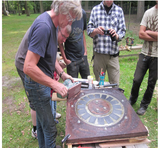
An electric sander was used to vibrate the moulds to get rid of air bubbles
