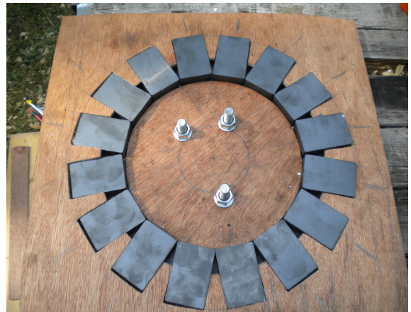
Magnets glued in the positioning jig
