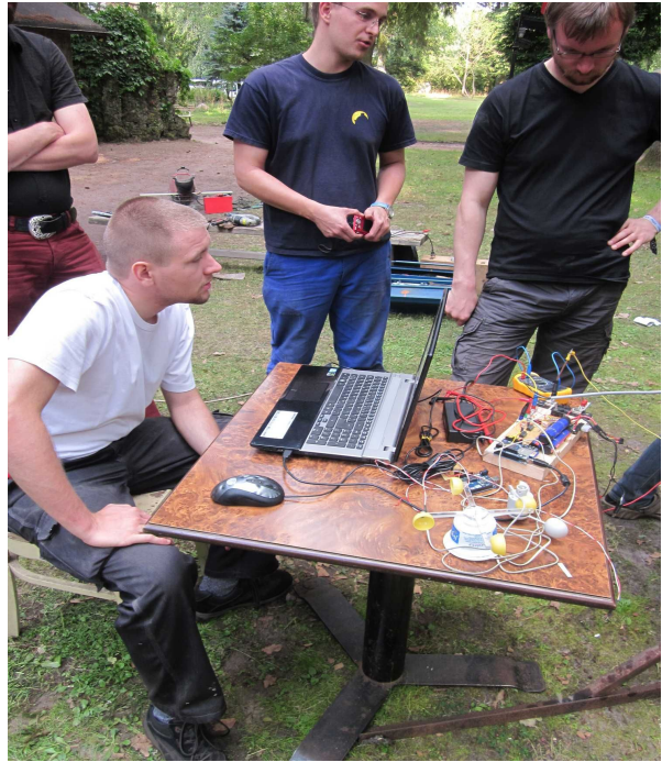
An Arduino System to measure output voltage and rpm
