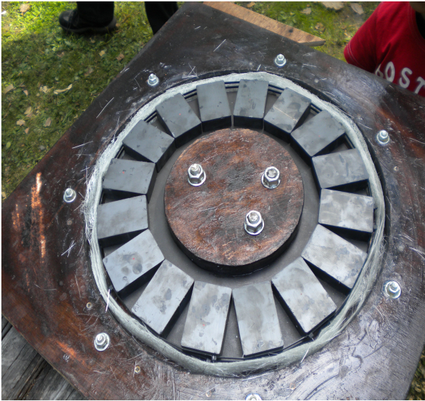
Magnets with a ring of cable ties and fibreglass ready for casting
