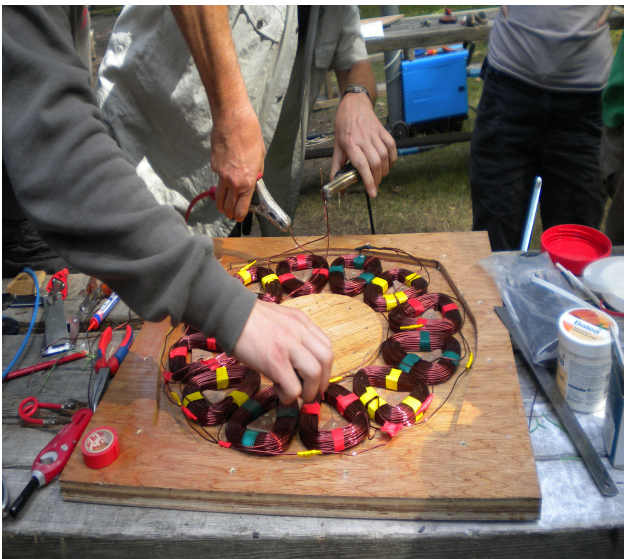
Coils positioned on the islands for soldering
