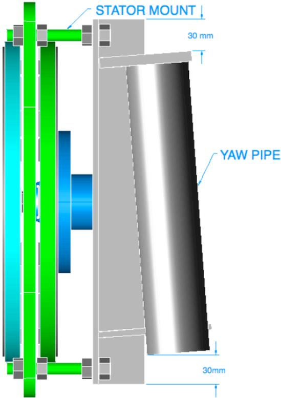
Next is to weld the brackets to the inside of the angle (piece 1) of the alternator frame. Position the yaw pipe centrally so that there is about 30 mm of angle projecting top and bottom.
