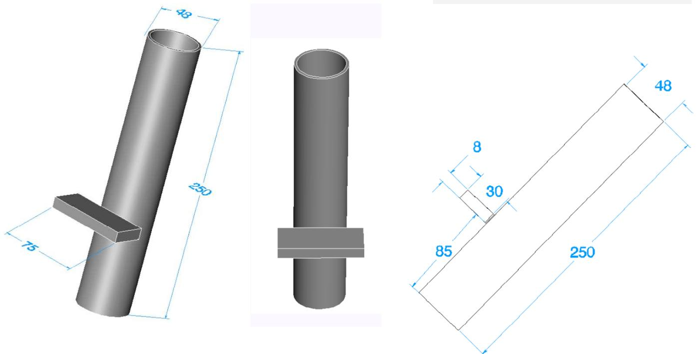
The next task is to set the frame of the turbine up at the correct angle so that this hinge pipe can be simply welded vertically above the yaw pipe.
