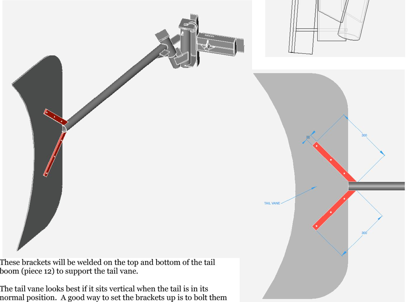
These brackets will be welded on the top and bottom of the tail boom (piece 12) to support the tail vane.
