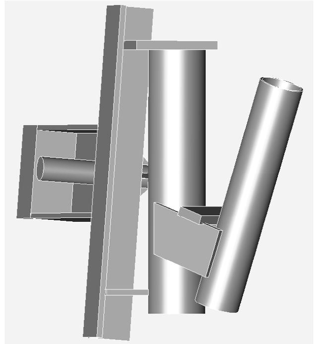
Piece 8 is the inner pipe of the hinge, 250 mm long.
