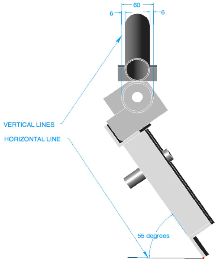
Clamp the two pipes together with vice-grips. The end of the hinge pipe should be welded to the yaw pipe about 20 mm from its end.
