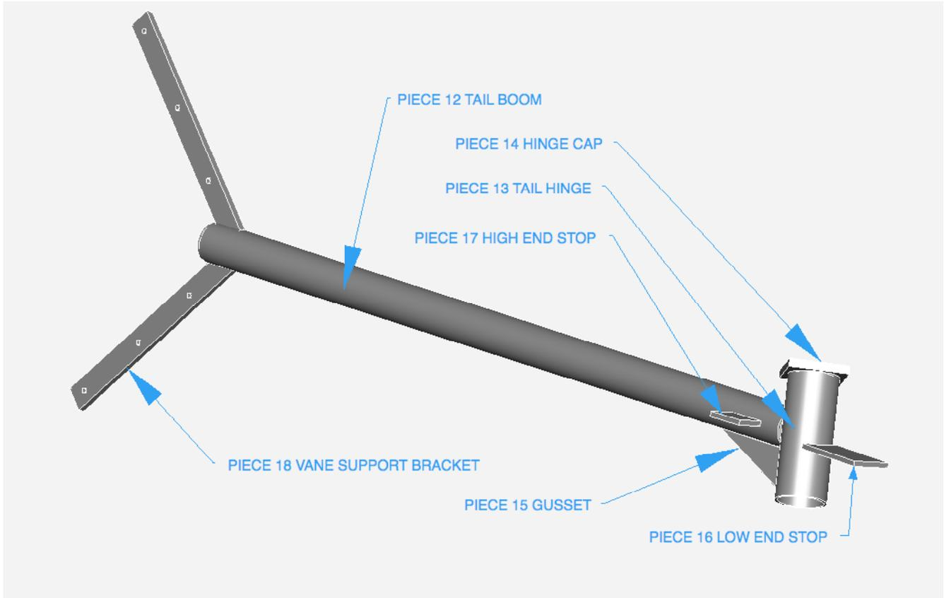
Start off by welding the cap onto the tail hinge pipe (pieces 13 and 14) . The hinge pipe (piece 13) is 150 mm length of 1 1/2" pipe.
