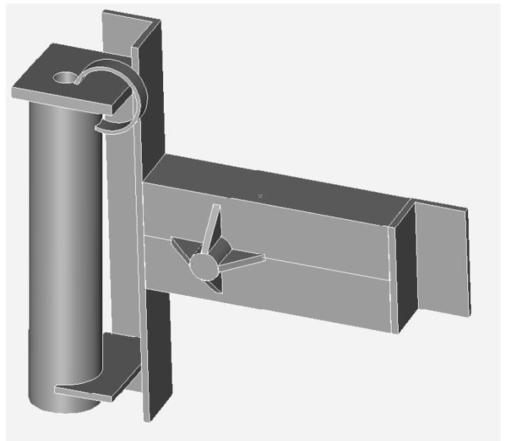
**6. When it is well positioned, weld the top (6) and bottom (7) brackets of the yaw pipe to the alternator frame (piece 1).**
