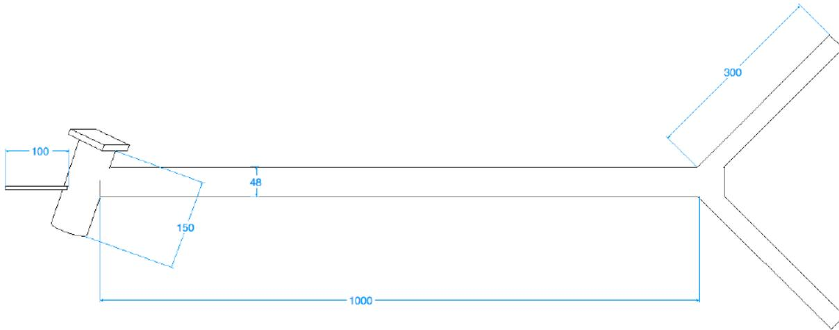
Cut the tail boom out of 1 1/2" pipe 1000 mm long. Measure a point 15 mm from the end of the boom and cut at 45 degrees as shown on the right.
