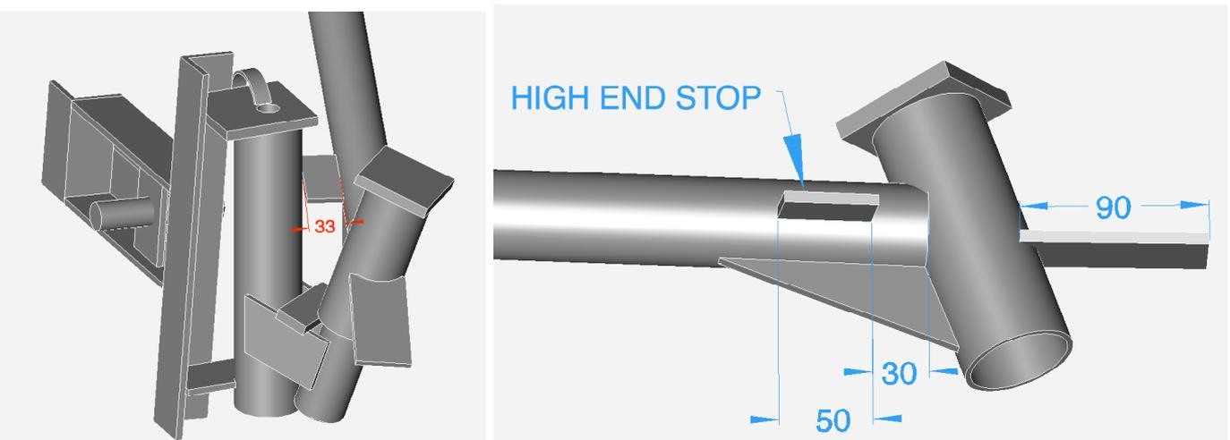
Cut out the high end stop (piece 17) 33 mm long. This is to be welded to the side of the tail boom such that it will contact the yaw pipe (piece 5) when the tail is lifted to its fullest extent.
