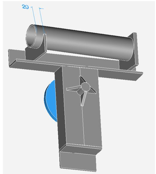
When preparing the stator to mount on the frame it will be useful to be able to drill the stator using the frame itself as a template. So allow enough clearance for a drill to pass through the frame from behind.
