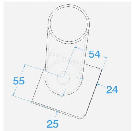
3. Mark the hole centre and draw the outline of the pipe (using a 30 mm radius on compasses) before drilling the hole.
