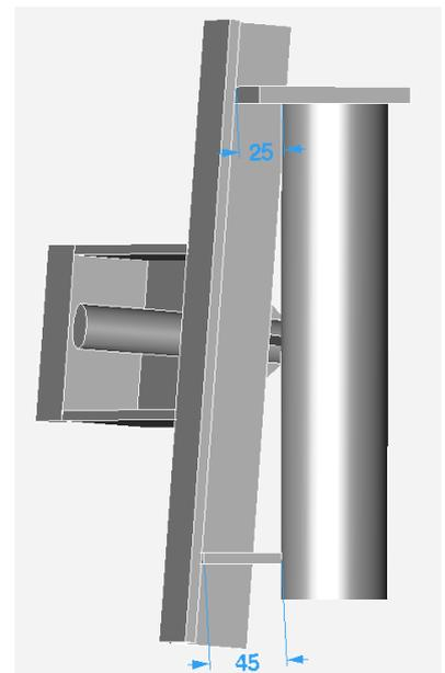
Again the exact overall size is not important. In this drawing it is 50 x 100 mm overall. The important measurements are again the clearances between the yaw pipe and the inside of the angle piece 1 to which it will be welded. If they were the same as those used for the cap then the frame would be parallel to the upright yaw bearing. Instead the lower bracket is 45 mm from the frame so as to kick it outward slightly, and create a 4 degree angle to the vertical.
