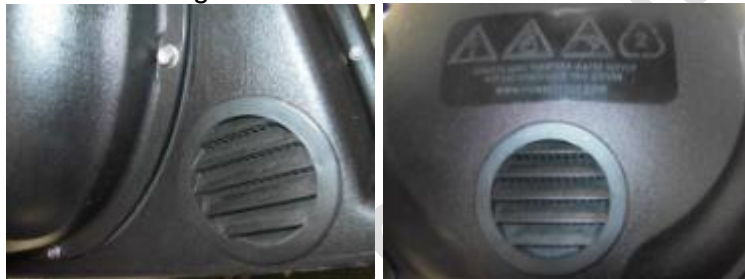
2 x side air vents and 1 x rear lid air vent – keep them clean
