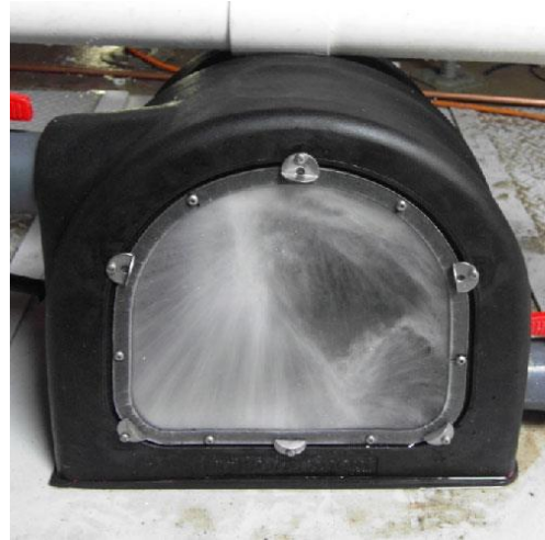
Top and bottom jet exhaust water is bouncing back towards the jet, indicating turbine is running slow. A little more magnetic rotor packing is needed.
