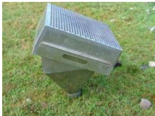
Some ideas for intakes made from scrap stainless steel components
