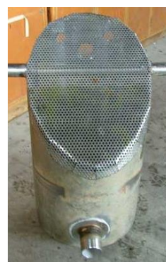
Some ideas for intakes made from scrap stainless steel components
