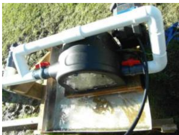
PowerSpout PLT200 running at 1500W
